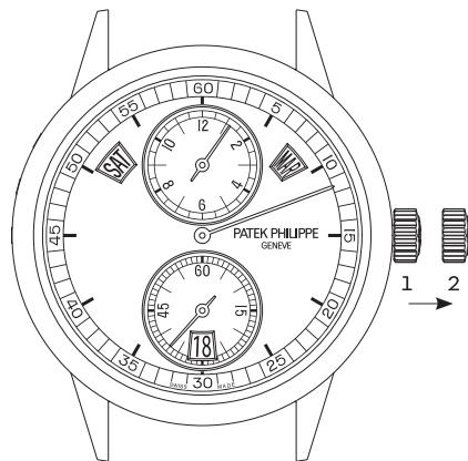
Your watch has a stop-seconds mechanism that halts the second hand as soon as you pull the crown out to position 2. This allows you to synchronize your watch with an acoustic time signal to one-second accuracy. As soon as you push the crown home (position 1), the second hand will start running again.
