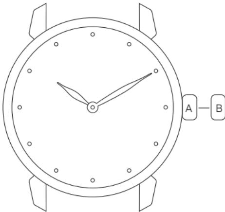
A Winding the movement: turn the crown clockwise.
