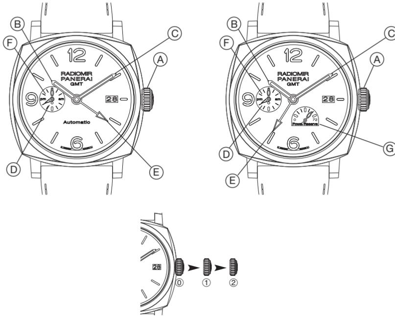
**(A) WINDING CROWN (B) HOURS (C) MINUTES (D) SMALL SECONDS
