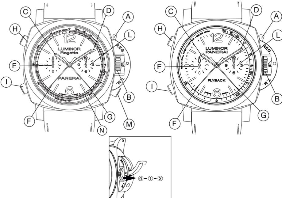
**(A) LEVER (B) WINDING CROWN (C) HOURS (D) MINUTES (E) SMALL SECONDS
