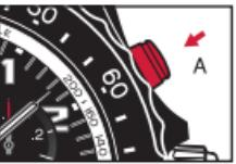
2. Stop the measurement by pressing pushpiece **A** once more. The measurement is made in hours [totalizer **1**], minutes [hand **2**], seconds [hand **3**] and  $\frac{1}{10}$ ths of a second [totalizer **4**].
