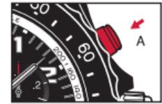
2. To interrupt the measurement, press pushpiece **A** once more. To restart the time measurement, press pushpiece **A**. This procedure makes it possible to add up several short times.
